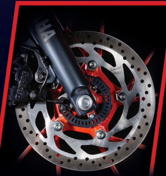
Single Channel ABS with 282(Fr)/220mm(Rr) Disc Brake
