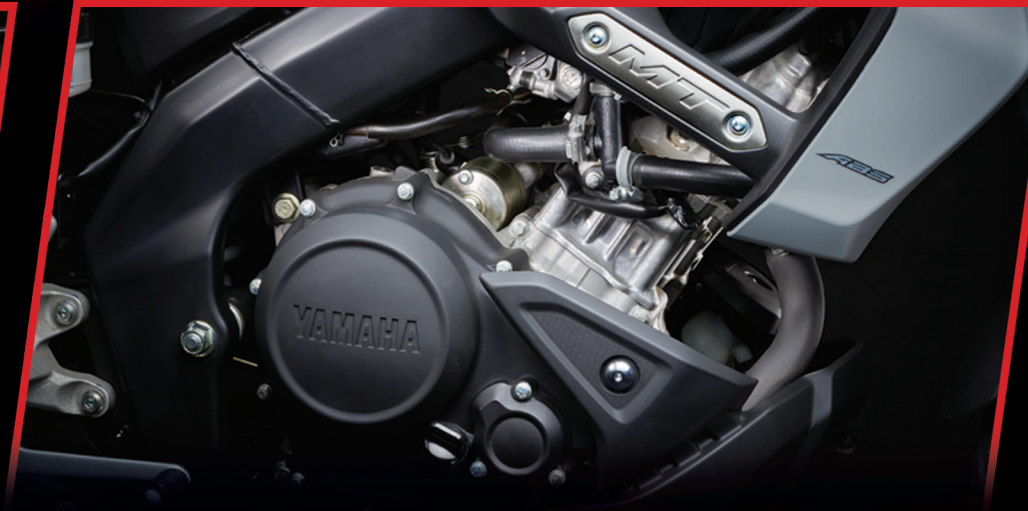
BS-VI Compliant 155cc LC4V SOHC Fuel Injection Engine
